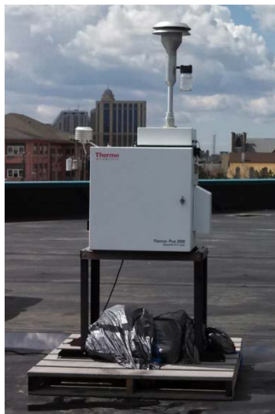
Figure 2 USEPA-Approved PM 2.5 Sampler in Atlantic City
